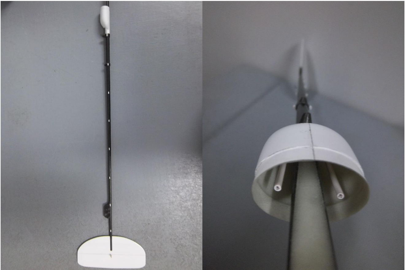
Picture 2.7. Pasting in the Bowden tubes
