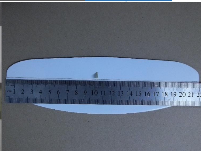
Picture 2.3. Pasting in the pylons of the elevating rudder
