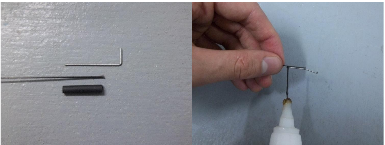
Picture 2.6. Pasting in the rod tip.
